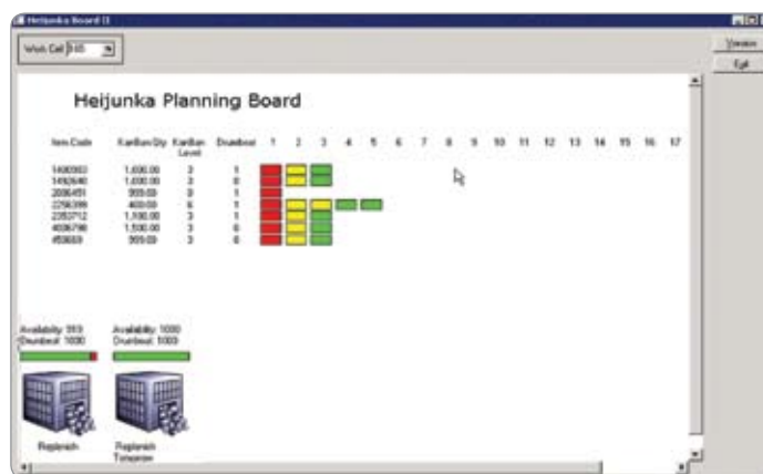
Level production and improve replenishment efficiency with tools such as the heijunka board and kanban stop/go board.
